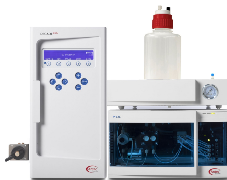
Figure 7. Dedicated ALEXYS FDG analyzer consisting of a DECADE Elite with SenCell Au- HyREF, P 6.1L isocratic pump, ET 210 eluent tray, manual injector and Clarity CDS for instrument control and acquisition.
